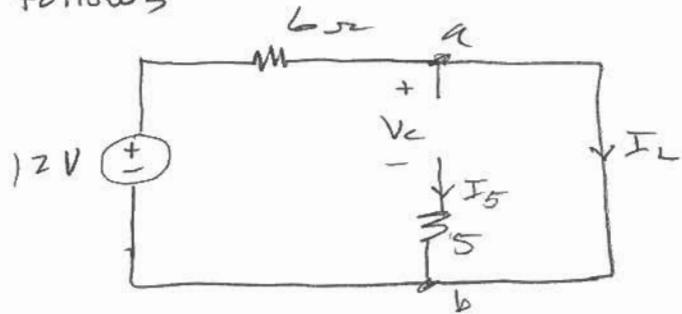
(a) By inspection, since  $I_5 = 0$  and  $V_{ab} = 0$ ,
