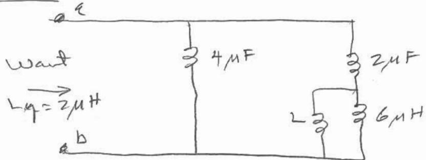
$$L_{eq} = \frac{6 \text{ mH} \times L}{L + 6 \text{ mH}} + 2 \text{ mH} = \frac{6L + 2L + 12}{6 + L}$$
