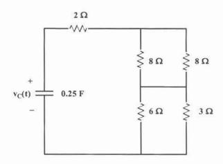
(5) You are given the circuit shown below. Use the differential equation technique to find  $v_C(t)$ .
