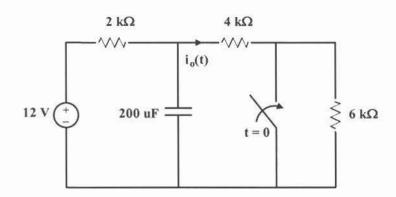
(8) The switch in the following circuit has been open for a very long time. It is closed at t = 0. Use the step-by-step technique to find  $i_0(t)$  for  $t \ge 0$ .
