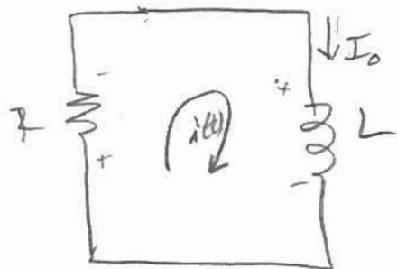
Figure 14.7: The unforced L-R circuit.
