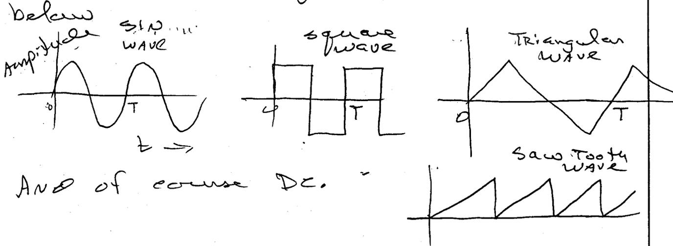
Why these waveforms? To start with, the sine wave is the fundamental waveform used in the power industry, worldwide. It is 60 Hertz (cycles/sec) in the US. In parts of Europe, maybe Japan it is 50 Hertz.
