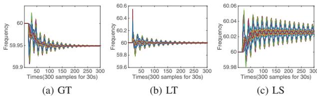
Fig. 2. Frequency signals on several buses (plotted in different colors) responding to the same single event.
