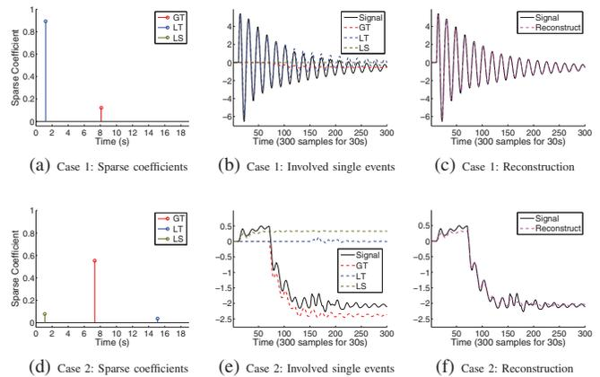
Fig. 9. Detection of unbalanced events: Case 1: ground truth is an LT occurred at the 1st sec and GT at the 8th sec; Case 2: ground truth is an LS happened at the 1st sec, a GT at the 7th sec, and an LT at the 15th sec.
