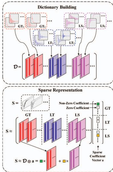
Fig. 7. Overview of the cluster-based sparse coding method. The top one: the diagram of dictionary building. The bottom one: the diagram of sparse representation.
