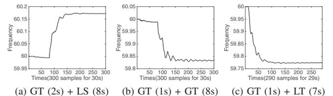
Fig. 5. Three cases with unbalanced events: (a) concatenated events with a small GT occurred at the 2nd sec and a large LS at the 8th sec; (b) concatenated events with small GT at the 1st sec and large GT at the 8th sec; (c) concatenated events with a large GT at the 1st sec and a small LT at the 7th sec.
