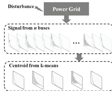
Fig. 6. Cluster-based signal extraction method for large power systems.
