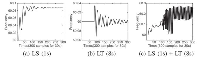
Fig. 4. Illustration of the nonlinear characteristic: (a) single event case: an LS occurred at the 1st sec; (b) single event case: an LT occurred at the 8th sec; (c) concatenated event with the same LS occurred at the 1st sec and the LT at the 8th sec
