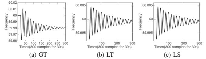
Fig. 3. Frequency signals display similar patterns responding to different single events.
