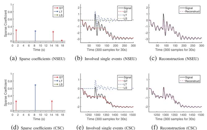
Fig. 10. Case 3: triple events case. The NSEU method detection result: a GT at the 1.16 sec, an LT at the 8.131 sec, a GT at the 14.64 sec, and GT at the 17.76 sec. The CSC detection result: a GT happened at the 1.113 sec, an LT at the 8.127 sec, and a GT at the 14.18 sec. The ground truth is a GT at the 1st sec, an LT at the 8th sec, and a GT at the 14th sec.
