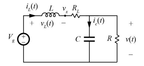
$$D = \begin{bmatrix} V_{g} & C & R_{L} & R & L \\ 1 & 0 & 0 & 0 & 1 \\ 0 & 1 & 0 & 1 & -1 \\ 0 & 0 & 1 & 0 & -1 \end{bmatrix} = \begin{bmatrix} I & D_{L} \end{bmatrix}$$
