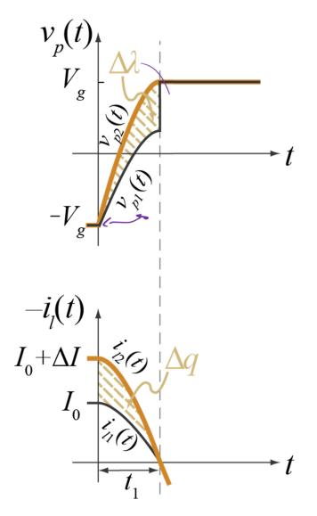
Solution different when partial hard switching occurs
