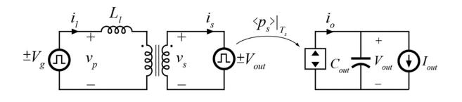
$$\langle i_o \rangle \Big|_{T_s} = \frac{V_{g/}}{n_t L_l T_s} \left( T_s t_{\varphi} - 2t_{\varphi}^2 \right)$$
