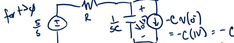
$$V_o(s) = \frac{5}{s} \left( \frac{\frac{1}{sC}}{R + \frac{1}{sC}} \right) + -(-C)(R \parallel \frac{1}{sC}) \rightarrow C \left( \frac{\frac{1}{sC}}{\frac{1}{R} + \frac{1}{sC}} \right) = C \frac{\frac{1}{sC}}{\frac{1}{RC} + s} = \frac{1}{\frac{1}{RC} + s}$$
