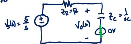
$$V_o(s) = V_{in}(s) \frac{Z_C}{Z_C + Z_R} = \frac{5}{s} \frac{\frac{1}{sC}}{\frac{1}{sC} + R} \rightarrow \frac{5}{s} \frac{\frac{1}{RC}}{\frac{1}{RC} + s}$$
