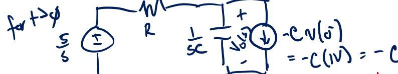
$$V_o(s) = \frac{5}{s} \left( \frac{\frac{1}{SC}}{R + \frac{1}{SC}} \right) + -(-c)(R || \frac{1}{SC}) \rightarrow C \left( \frac{\frac{1}{R}}{\frac{1}{RC} + SC} \right) = C \frac{\frac{1}{R}}{\frac{1}{RC} + s} = \frac{1}{RC + s}$$
