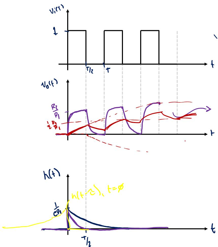
$$f_a(t) = \frac{R_2}{R_1} \left[ 1 - e^{-\frac{1}{R_2 C} t} \right] u(t)$$
