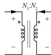
$$\frac{V_1(s)}{N_1} = \frac{V_2(s)}{N_2}$$
