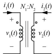
$$\frac{v_1(t)}{N_1} = \frac{v_2(t)}{N_2}$$
