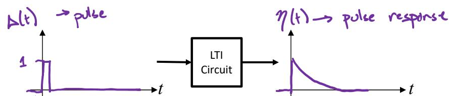
$$v_i(t) = \sum_{k=0}^{\infty} \Delta(t-kT) v_i(kT) \quad \text{by superposition}$$
