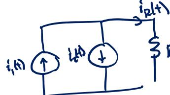
$$i_1(t) = I_{A1} \cos(\omega_1 t) \quad i_2(t) = I_{A2} \cos(\omega_2 t), \quad \omega_1 \neq \omega_2$$
