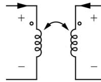
$$V_1(s) = sL_1 I_1(s) - L_1 i_1(0^-) + sM I_2(s) - M i_2(0^-)$$
