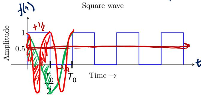
$$\text{period : } T_0 = \frac{1}{f_0} = \frac{2\pi}{\omega_0} \quad \omega_0 T_0 = 2\pi$$
