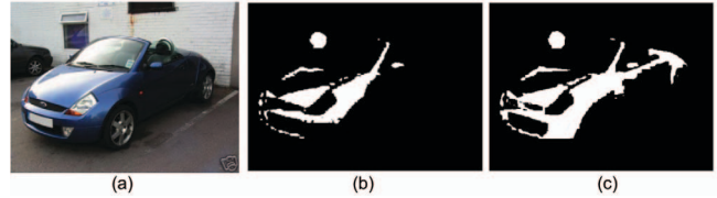
Fig. 3. The improvement gained when performing image level recognition using graph cuts. (a) Original image. (b) Pixels classified as blue before running the graph cut algorithm (Sec. 3.2). (c) Pixels classified as blue after using graph cuts. As can be seen the many of the holes that were not classified as blue in (b) because of lighting conditions were captured correctly in image (c) by using neighboring pixels.
