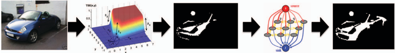
Fig. 2. An overview of our color classification method. Given an image we use Parametric Fuzzy Sets to classify each pixel to a color. We use the graph cuts to reduce the noise and achieve a more accurate color classifier.
