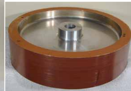
Drum Memory from a Bendix G-15 Computer (3" x 12.5")
