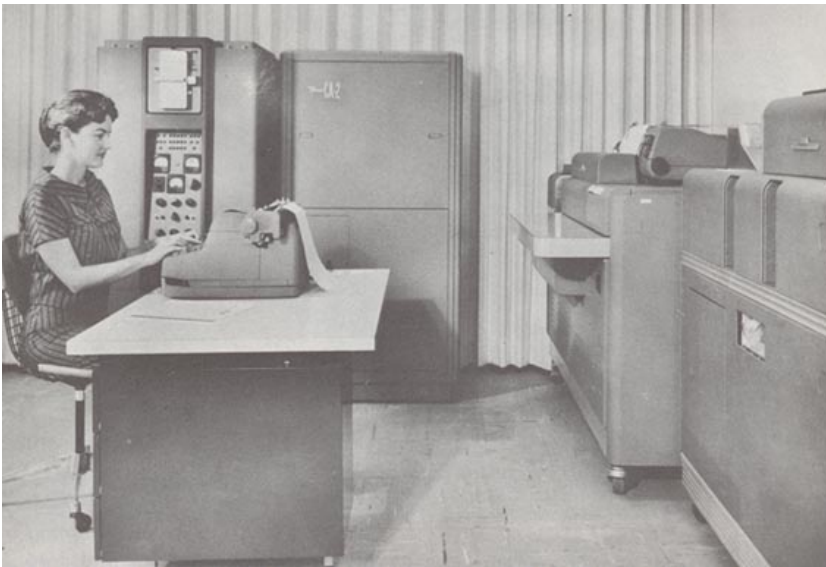
2160 words in 20 channels of 108 words each. Avg. access time 14.5 ms Note IBM peripherals. Monthly rental $1485.00 Purchase $49,500
