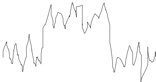
Figure II.2: Depiction of 0-1-0 pulses in the presence of high thermal noise.
