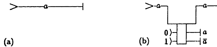
Figure II.15: The “spy circuit” for tapping into the output. Note that in the diagram the 0 and 1 constant inputs are switched (or, equivalently, the a and \bar{a} outputs are switched). [fig. from FT82]
