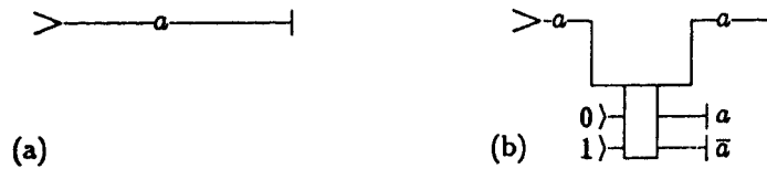
Figure II.18: The “spy circuit” for tapping into the output. Note that in the diagram the 0 and 1 constant inputs are switched (or, equivalently, the a and \bar{a} outputs are switched). See also the FAN-OUT circuit in Fig. II.15. [fig. from Fredkin & Toffoli (1982)]
