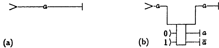
Figure II.19: The “spy circuit” for tapping into the output. Note that in the diagram the 0 and 1 constant inputs are switched (or, equivalently, the a and \bar{a} outputs are switched). See also the FAN-OUT circuit in Fig. II.16. [fig. from Fredkin & Toffoli (1982)]
