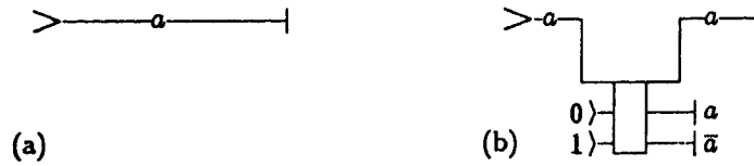
Figure II.18: The “spy circuit” for tapping into the output. [fig. from Fredkin & Toffoli (1982)]
