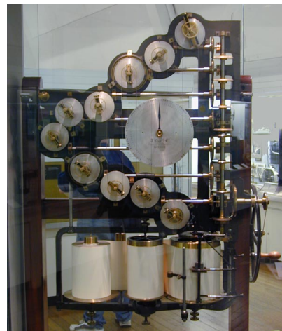
Figure V.8: Lord Kelvin’s analog tide computer. [source: wikipedia]
