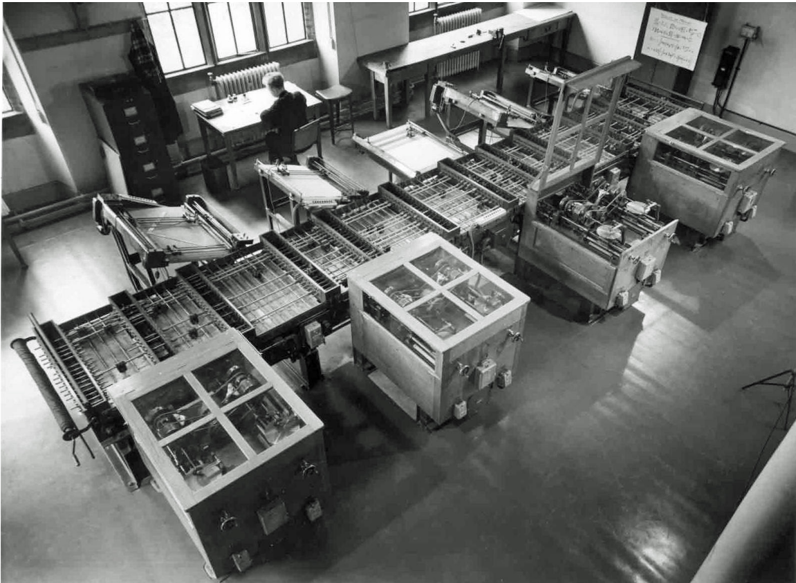
Figure V.9: MECCANO differential analyzer at Cambridge University, 1938. The computer was constructed by Douglas Hartree based on Vannevar Bush's design. [source: wikipedia]
