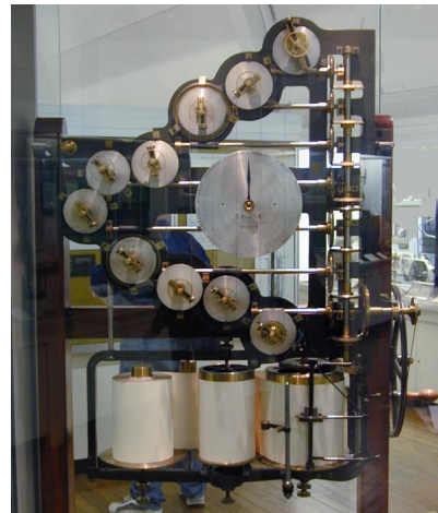
Figure V.8: Lord Kelvin’s analog tide computer. [source: wikipedia]
