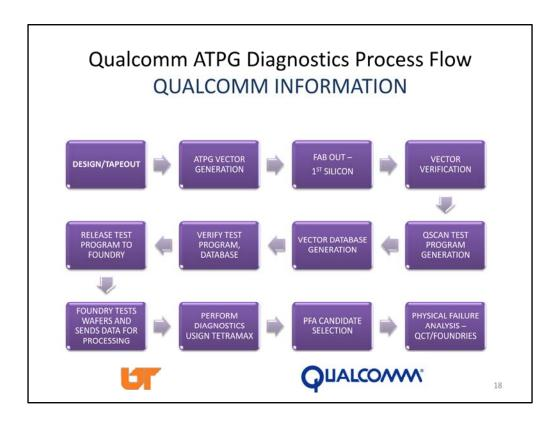
The details included in this slide and the following slides describe the procedure used by Qualcomm. This slide shows a sequence of steps that leads to ATPG diagnostics and the post processing steps that follow.
