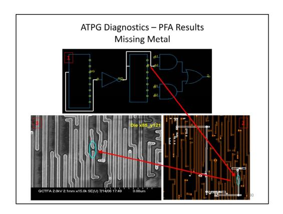
Another example is shown here where a metal line has a small piece of metal missing. This could be due to a small impurity that could have been introduced during the fabrication process exactly at this step.
