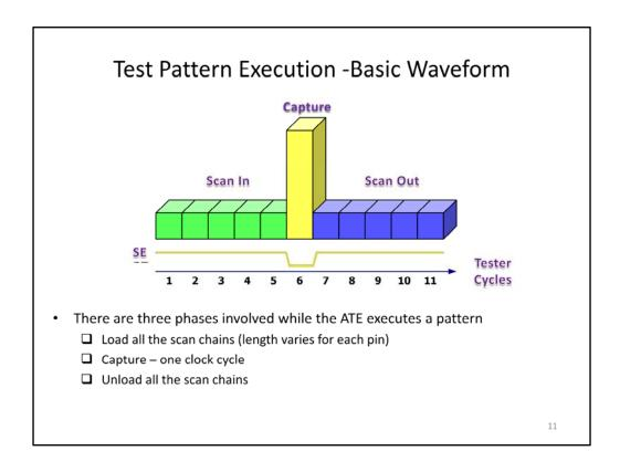
This slide is a graphical representation of the various stages that are required by a tester to execute a pattern. In the previous example, a 5-bit scan chain was considered, so it takes 5 tester cycles to load and unload each pattern. It takes one tester cycle for the ATE to perform the capture procedure, (force the PIs and observe the POs). A detailed explanation is included in the previous slide.
