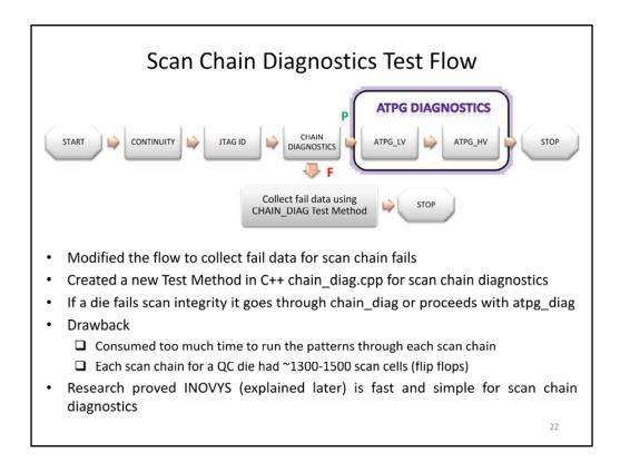
This slide explains how I created a tool to capture FAIL data for scan chain integrity fails. This test method called CHAIN\_DIAG.cpp used a similar flow, but it was modified to treat the scan chain integrity fails differently. The basic idea behind this test method is as follows.
