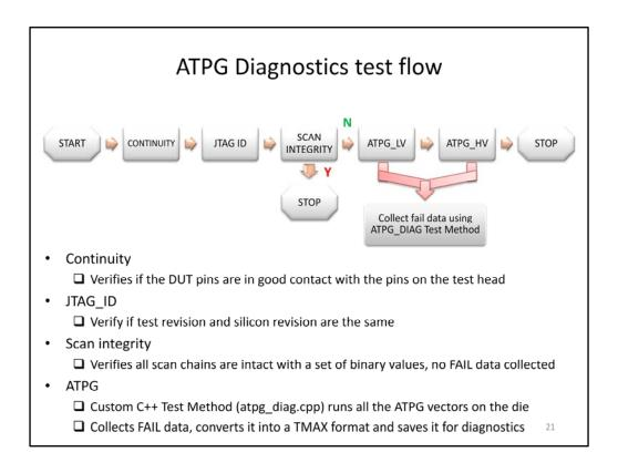
The test flow used to perform ATPG diagnostics and collect FAIL information is explained in this slide. The test flow consists of test suites to perform the following functions.
