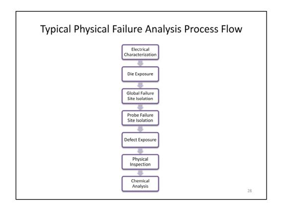
This slide explains each step followed in a typical failure analysis flow.
