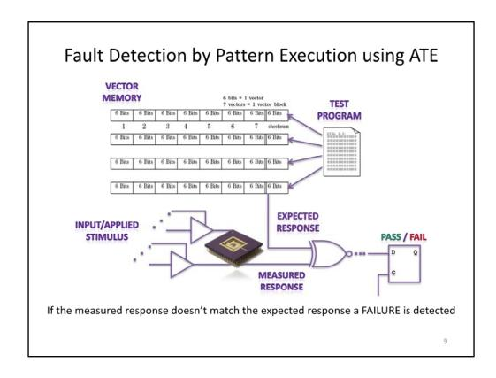
This slide explains how a fault detection is implemented by the ATE hardware. The basic criterion is that a fault is detected by an applied input if the measured output doesn't match the expected response. This is a conceptual diagram using differential comparators to detect the differences between the responses, if any.
