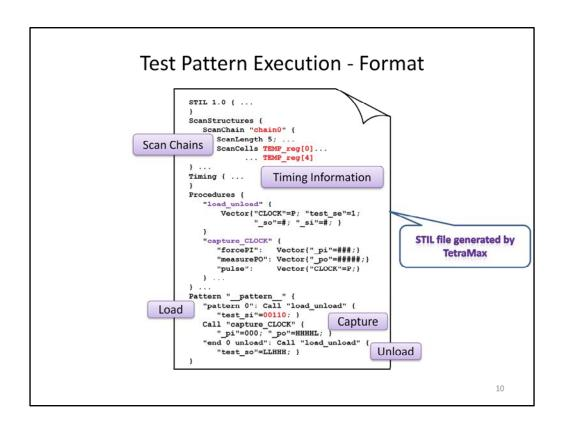
This slide explains how TetraMax creates the patterns and dumps them (writes out) into a STIL file. This is an example of an executable STIL file generated by TetraMax. STIL stands for standard test interface language and it is an industry standard. It encompasses a tester description of test patterns, pin timing protocol and scan paths. This example STIL files show how user procedures are created to concisely describe repetitive actions. Let us consider an example of a 5-bit scan chain chain 0.
