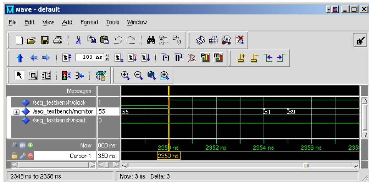
**18. Capture** the waveform and note the signal begins to change at 2354 ns and stabilizes at 2355 ns instead of 2250 ns for a delay of **5 ns** + 100ns (initialization).
