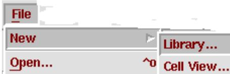
13. Then, select File→New→Cell View and fill in “inverter” & “schematic”
