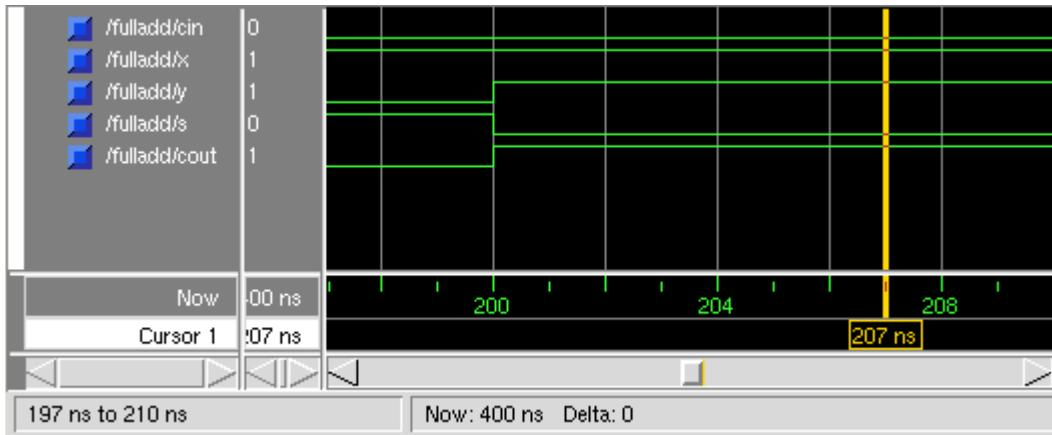
Note that the inputs and outputs both change instantly at 200 ns.
