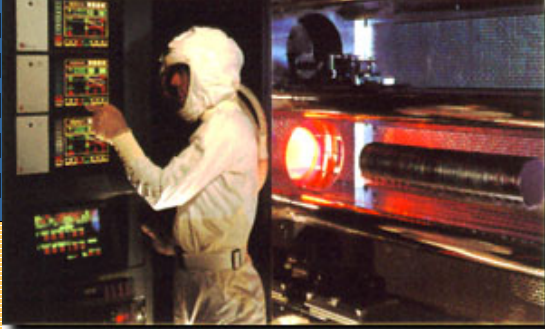
Oxidation Furnace (Silicon Valley Group - Thermco Systems)
