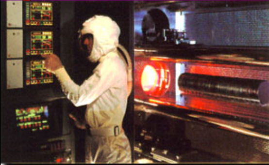
Oxidation Furnace (Silicon Valley Group - Thermco Systems)
