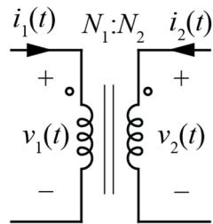
$$\frac{v_1(t)}{N_1} = \frac{v_2(t)}{N_2}$$
