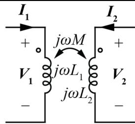
$$\underline{V}_1 = j\omega L_1 \underline{I}_1 + j\omega M \underline{I}_2$$
