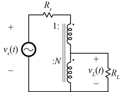
Find  $v_L(t)$  for  $v_s(t) = 170\cos(2\pi 60t)$  and for  $R_s = 10 \Omega$ ,  $N = 0.1$ , and  $R_L = 50 \Omega$
