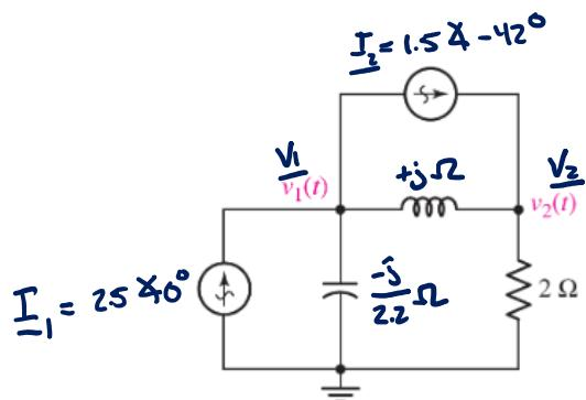
By superposition, with  $\underline{I}_1$  on
