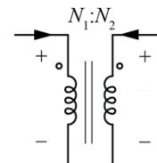
$$\frac{V_1(s)}{N_1} = \frac{V_2(s)}{N_2}$$
