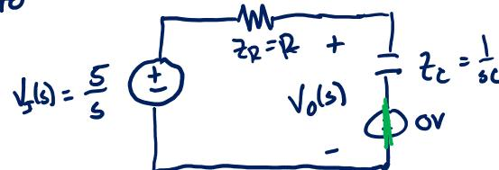
$$v_o(s) = V_I(s) \frac{\frac{1}{sC}}{\frac{1}{sC} + R} = \frac{5}{s} \frac{\frac{1}{sC}}{\frac{1}{sC} + R} \rightarrow \frac{5}{s} \frac{\frac{1}{RC}}{\frac{1}{RC} + s}$$
