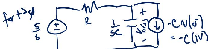
$$v_o(s) = V_I(s) \frac{\frac{1}{sC}}{\frac{1}{sC} + R} + C(V) \left[ R \parallel \frac{1}{sC} \right]$$
