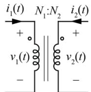
$$\frac{v_1(t)}{N_1} = \frac{v_2(t)}{N_2}$$
