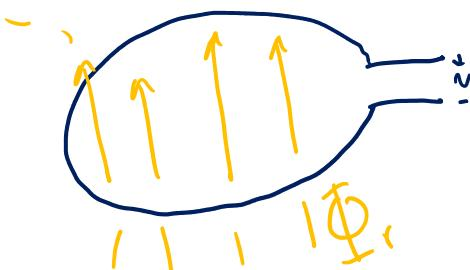
$$V_1 = N \frac{d\Phi}{dt}$$
