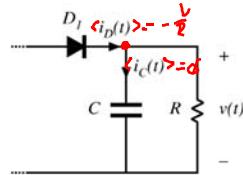
must compute dc component of diode current and equate to load current (for this boost converter example)
