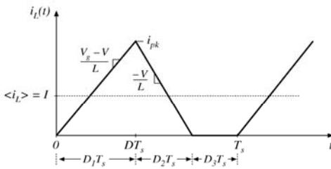
equate dc component to dc load current:
