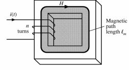
For uniform field strength H(t), the core MMF around the path is  $H \ell_w$ .
