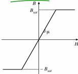
Typical  $B_{sat} = 0.3$  to 0.5T, ferrite 0.5 to 1T, powdered iron 1 to 2T, iron laminations
