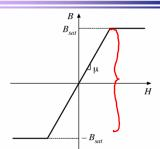
Find winding current at onset of saturation: substitute  $i=I_{sat}$  and  $H=B_{sat}/\mu$  into equation previously derived via Ampere's law. Result is
