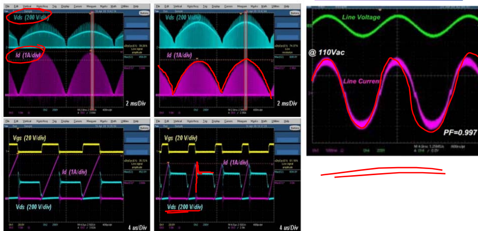
(a) at 110 V ac Input (b) at 220 V ac Input Figure 12. Switching Voltage and Current
