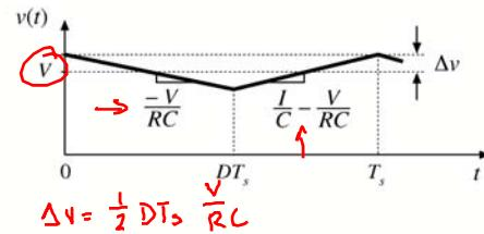
Change in capacitor voltage during subinterval 1 is (slope) (length of subinterval):
