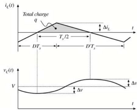
The total charge  $q$  is the area of the triangle, as shown:
