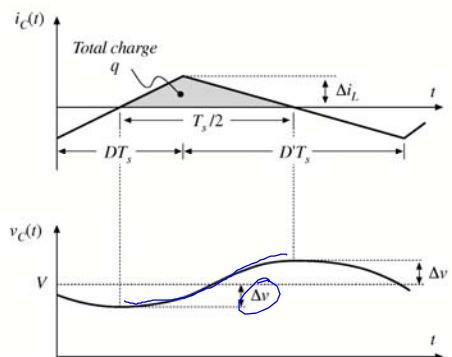
Current  $i_c(t)$  is positive for half of the switching period. This positive current causes the capacitor voltage  $v_c(t)$  to increase between its minimum and maximum extrema. During this time, the total charge  $q$  is deposited on the capacitor plates, where
