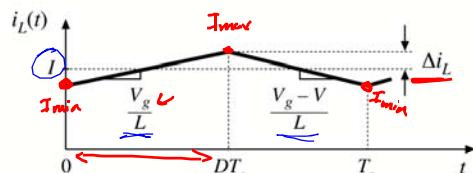
Change in inductor current during subinterval 1 is (slope) (length of subinterval):
