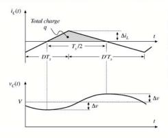
Current  $i_{c}(t)$  is positive for half of the switching period. This positive current causes the capacitor voltage  $v_{c}(t)$  to increase between its minimum and maximum extrema. During this time, the total charge q is deposited on the capacitor plates, where
