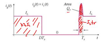
$\langle i_{g} \rangle = I_{g} = (area \ under \ curve)/T_{s}$
