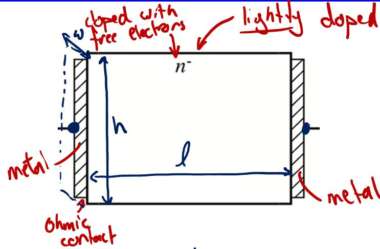
When conducting current through semiconductor
