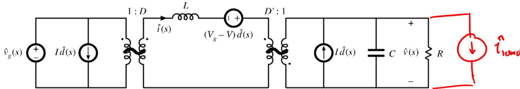
$$G_{vd}(s) = \left( -\frac{V_g - V}{D'} \right) \frac{1 - sL \frac{I}{D'(V_g - V)}}{1 + \frac{sL}{D'^2 R} + s^2 \frac{LC}{D'^2}}$$
