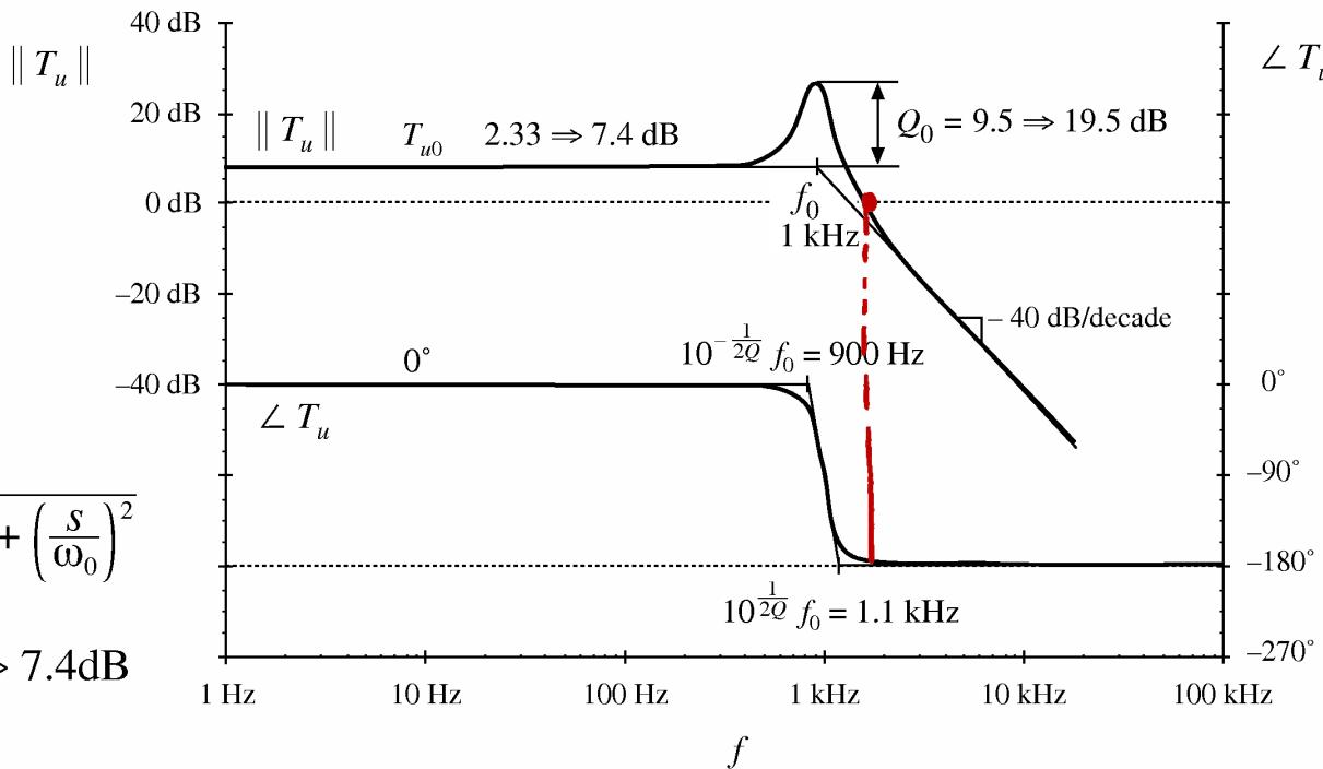
$$f_c = 1.8 \text{ kHz}, \varphi_m = 5^\circ$$
