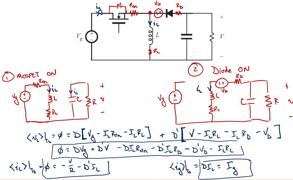
Equivalent Circuit Model  $\phi = DV_0 - DV_1 - DV_2 - DV_3 - DV_4 - DV_5 - T_1 R_1$   $\phi = DV_0 - DV_1 - DV_2 - DV_5 - DV_5 - T_1 R_1$   $\phi = DV_0 - DV_1 - DV_2 - DV_5 - DV_5 - T_1 R_1$ 0 = - N - D'IL P.:1 1:D PL DRUN D'RD
