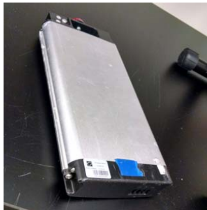
10Ah Li-ion ~26V battery
