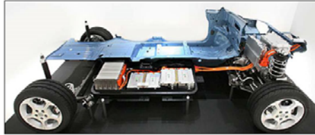
Cutaway battery of Nissan Leaf electric vehicle. The Leaf includes a 24kWh lithium-ion battery with a city driving range of 160km (100 miles). The battery fits under the floor of the car, weighs 272kg (600lb) and is estimated to cost $15,600 (2010).
