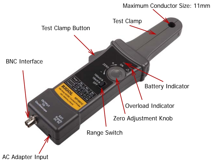
Figure 1 RP1001C Current Probe
