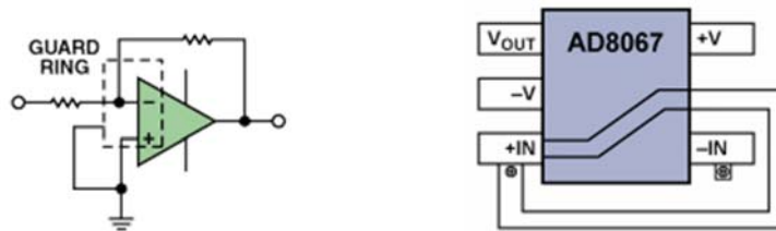
Figure 12.26: An Operational Model of a Faraday Shield
