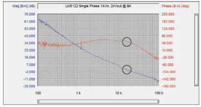
$F_C \sim 15 \text{ kHz}$ ; PM  $\sim 50^{\circ}$
