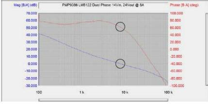
$F_C \sim 7.5 \text{ kHz}, PM \sim 60^{\circ}$
