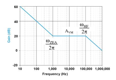
$$\frac{\omega_{\text{ZEA}}}{2\pi} = \frac{\omega_{\text{C}}}{2\pi \times 10}$$
