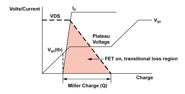
$$SW_{TRANSLoss} = Vout \times I_{in\_Avg} \times T_{SLEW} \times F_{SW}$$
