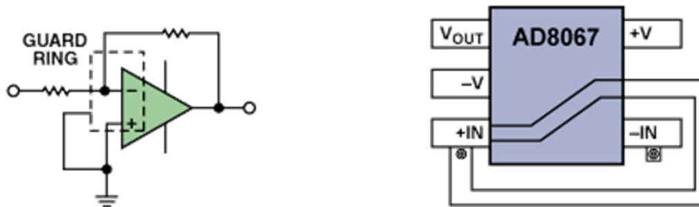
Figure 12.26: An Operational Model of a Faraday Shield
