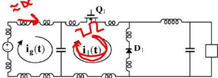
high frequency currents are shunted through capacitor instead of input source
