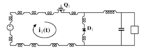
Addition of bypass capacitor confines the pulsating current to a smaller loop:
