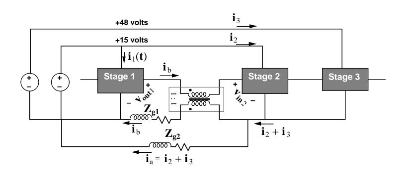
The common-mode choke forces the high frequency return current  $(i_2 + i_3)$  to flow through the alternate ground path:  $i_a = (i_2 + i_3)$ . The return current  $i_b$  is equal to the signal current flowing between stages 1 and 2.
