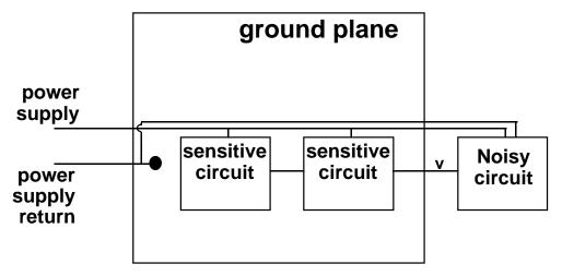
A solution is to remove the noisy circuit from the ground plane. One could then run a separate ground wire for the noisy circuit. The only drawback is that noise can be coupled into the input signal v.
