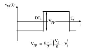
The secondary ground potential switches at high frequency with respect to the primary ground.
