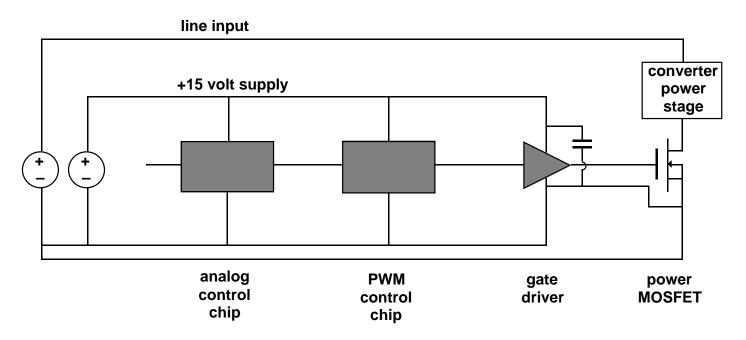
High frequency components of gate drive current are confined to a small loop
