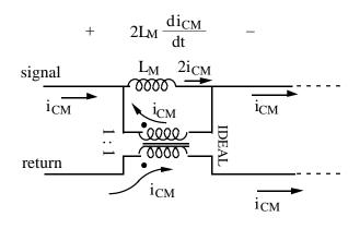
The common-mode currents effectively add, magnetizing the core. The common-mode choke presents inductance  $L_{\rm M}$  to filter these currents.
