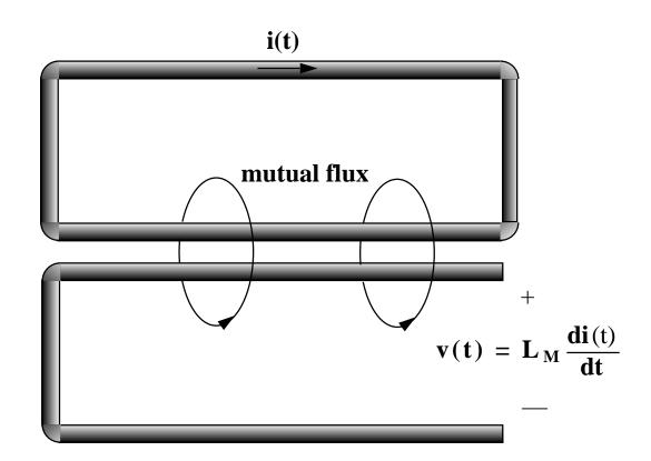
This phenomenon can sometimes be a problem when ground loops are present. Circulating ground currents are then induced, which lead to variations in the ground reference potential
