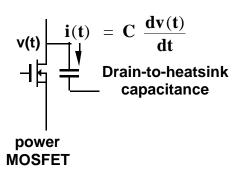
When the switched drain voltage is applied to this capacitance, current spikes must flow.
