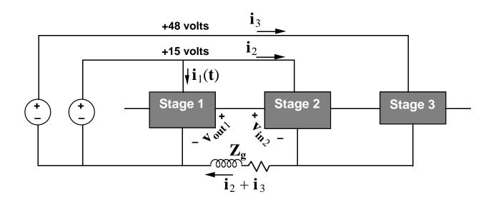
$$\mathbf{v_{in2}} = \mathbf{v_{out1}} - \mathbf{Z_g} (\mathbf{i_2} + \mathbf{i_3})$$
