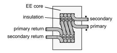
A simple lumped element model, including interwinding capacitance:
