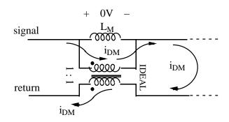
i<sub>DM</sub> cancels out in windings, with no net magnetization of core. To the extent that the leakage inductance can be neglected, the commonmode choke has no effect on the differential-mode currents.
