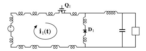
Addition of bypass capacitor confines the pulsating current to a smaller loop:
