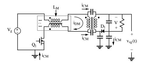
Common-mode choke inserts inductance  $L_{\rm M}$  to oppose flow of high-frequency common-mode currents
