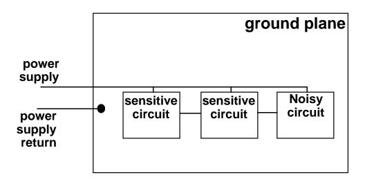
Return current of noisy circuit runs underneath sensitive circuits, and can still corrupt their ground references
