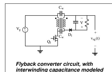
One can solve the circuit to find the high-frequency ac component of  $v_{sg}(t)$ . The result is
