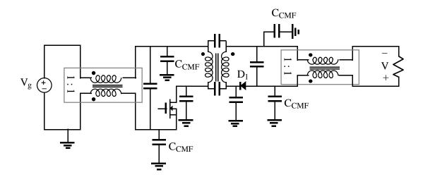
The common-mode chokes, along with the capacitors  $C_{\text{CMF}}$ , form two-pole low pass filters which oppose the flow of high-frequency common-mode currents
