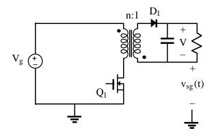
Transformer interwinding capacitance causes currents to flow between the isolated (primary and secondary) sides of the transformer, and can cause the secondary-side ground voltage to switch at high frequency: v<sub>sg</sub>(t) contains a high-frequency component.
