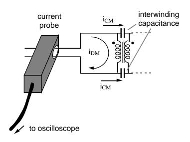
The common mode current due to transformer interwinding capacitance can be easily measured using a current probe
