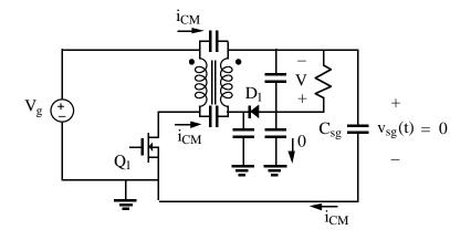
Capacitor  $C_{sg}$  is much larger than the stray capacitances, and so nearly all of the common-mode current flows through  $C_{sg}$ . If  $C_{sg}$  is sufficiently large, then it will have negligible voltage ripple, and  $v_{sg}(t)$  will no longer contain a high-frequency component.
