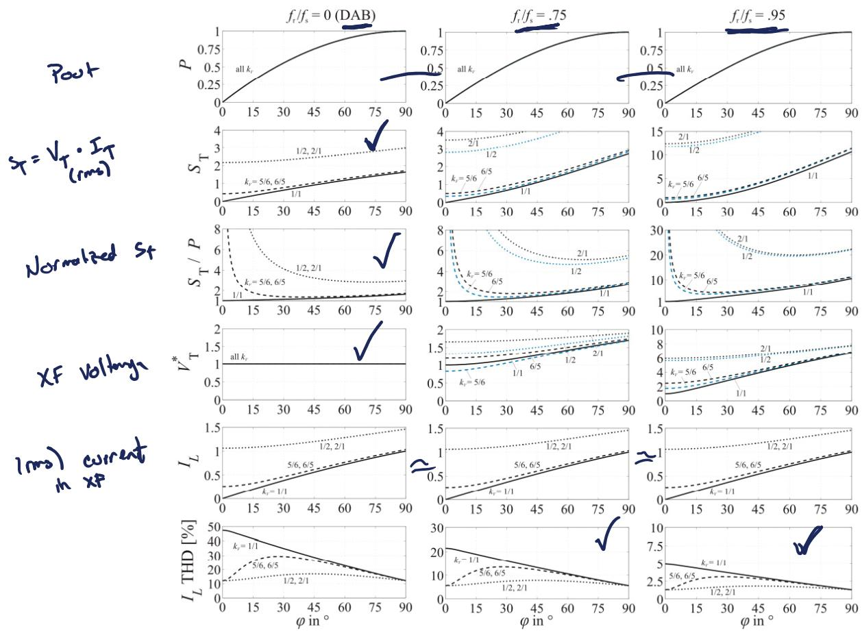
R. Lenke, F. Mura and R. W. De Doncker, "Comparison of non-resonant and super-resonant dual-active ZVS-operated high-power DC-DC converters,"
