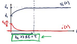
$$\Delta E_{c} = \frac{1}{2} C V_{2}^{2} - \frac{1}{2} C V_{1}^{2}$$
