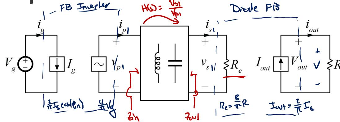
For FB Inverter, FB Diode Rectifier
