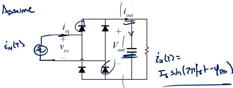
$$V_{s1}(t) = \frac{4}{\pi} V_{out} \sin(2\pi f_s t - \phi_{ps})$$
