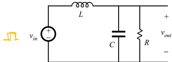
$$\|H(s)\| = \frac{|v_{out}|}{|v_{in}|} = \frac{1}{s^2 LC + s \frac{1}{R} + 1} = \frac{1}{(\frac{s}{\omega_0})^2 + \frac{2}{Q\omega_0}s + 1}$$
